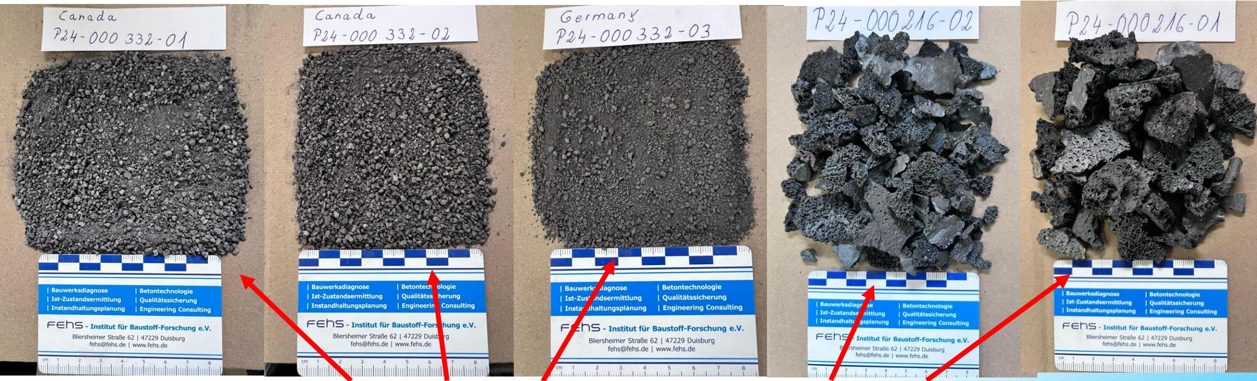
In total >10 different EAF slag samples, with DRI as iron carrier from 10-95 %, were collected from all over the world and characterized
