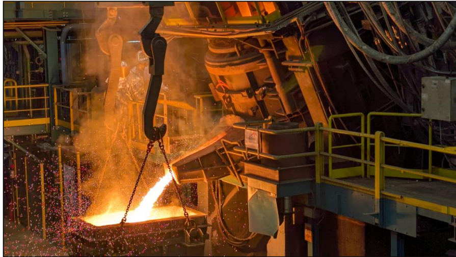
Slag is generated in our 6-ton pilot (≈300/400 kg of slag)
